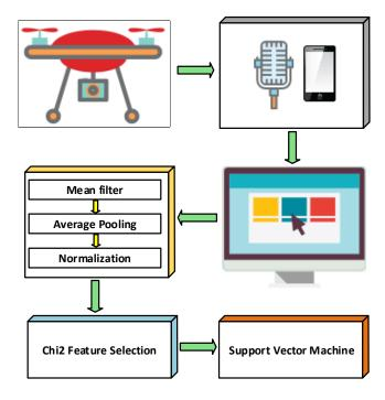
Fig. 3. Block diagram of the proposed method
