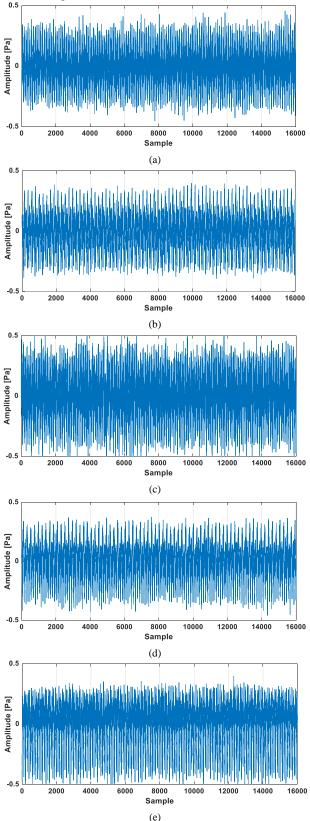
Fig. 2. Sound samples collected for fault detection (a) Healthy, (b) Balance Failure, (c) Magnet Failure, (d) Propeller Failure, (e) Bearing Failure
